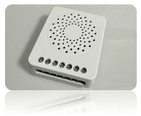
This is a radio transmitter that activates in the presence of an electric current. In a hotel, it is useful for monitoring water flow in unoccupied rooms.
